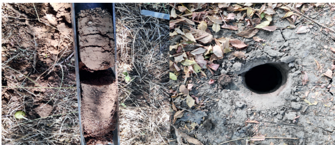
Fig. 7. Sample collection by soil core method to assess bulk density
