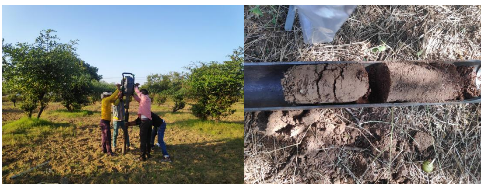
Fig. Soil sampling rig used for soil collection from agroforestry system
