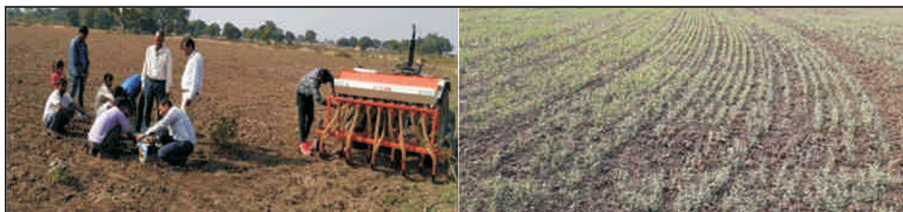
Plate 23A: Sowing using a zero-tillage multicrop planter after laser levelling in Jhansi
